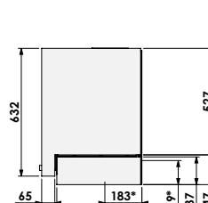
\* Optional flue gas outlet Ø 130 mm
