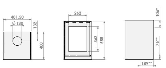
\* Optional flue gas outlet Ø 130 mm
