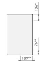
\* Optional flue gas outlet Ø 150 mm
