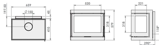
\* Optional combustion air supply Ø 125 mm
