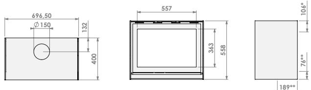
\* Optional flue gas outlet Ø 150 mm
