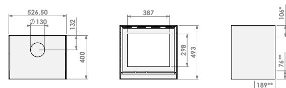
\* Optional flue gas outlet Ø 130 mm
