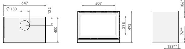
\* Optional flue gas outlet Ø 130 mm
